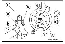
• Fit the pin [A] of the oil pump cover [B] into the hole [C] in the crankcase.
