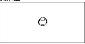
Valve Seat Cutter,  $60^{\circ}$  - $\phi$ 27: 57001-1409
