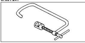
Piston Pin Puller Assembly: 57001-910
