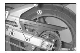
Disengage the drive chain [A] from the engine sprocket [B], and take it off the chassis.
