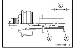
• Set the fork spring compressor on the washer using the outer tube as a guide.
