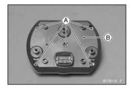
• Separate the meter liquid crystal display assembly [A] and upper meter cover [B].
