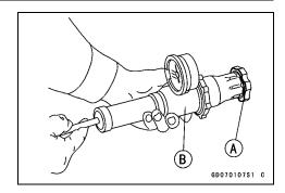
Watching the pressure gauge, pump the pressure tester to build up the pressure until the relief valve opens: the gauge hand flicks downward. Stop pumping and measure leak time at once. The relief valve must open within the specified range in the table below and the gauge hand must remain within the same range at least 6 seconds.
