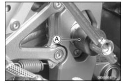
• Unscrew the swingarm pivot shaft nut [A].
