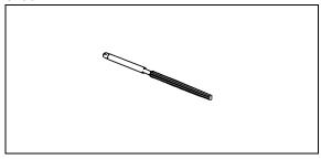
Valve Seat Cutter Holder, $\phi$ 4: 57001-1275
