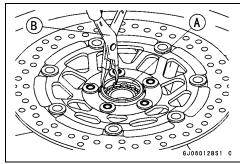
Use the bearing remover to remove the hub bearing [A].
