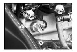
Radiator Fan Switch, Water Temperature Sensor Installation
