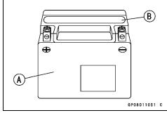
Terminal Voltage: 11.5 ~ less than 12.8 V Standard Charge 0.9 A × 5 ~ 10 h (see following chart) Quick Charge
