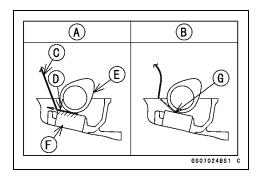
OWhen positioning #1 piston TDC at the end of the compression stroke:
