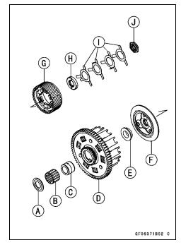
OInstall the spacer [A] so that the stepped side [B] faces inward.
