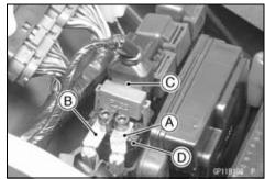
• Connect the hand tester [A] and 12 V battery [B] to the starter relay [C] as shown.
