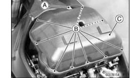
Install a new element [A] with the mesh side facing upward.
