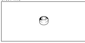
Valve Seat Cutter Holder Bar: 57001-1128
