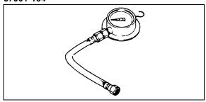
Oil Pressure Gauge Adapter, M18 × 1.5: 57001-1278
