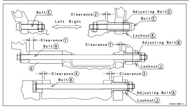
• Turn the adjusting bolt [A], [B] until the clearance [X], [Y] between the crankcase and frame come to zero mm (zero in.).
