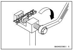
• Set plate holder (B) [A] and cutting and riveting pin [B] as shown.
