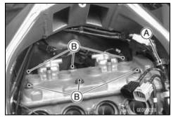
Remove the cylinder head cover [A] to backward [B] floating it a little up.
