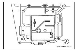
• Install the breather plate [B], and apply a non-permanent locking agent to the threads and tighten the bolts [A].
