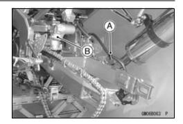
• Unscrew the swingarm pivot shaft locknut using socket wrench [A].
