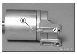
• Align the hollow mark [A] on the left-hand end cover and the hollow mark [B] on the yoke.
