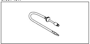
Valve Seat Cutter, 60° - $\phi$ 25: 57001-1328
