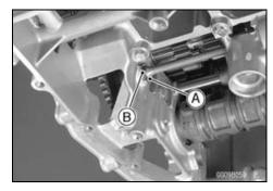
• Pull the oil pump drive gear [A].
