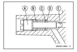
Back out the same number of turns counted when first turned in. This is to set the screw to its original position.
