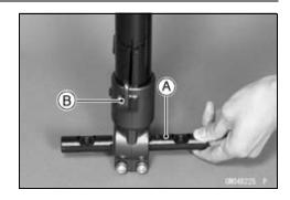
• Insert the compression shaft [A] with the 120 mm - thread length end upside, and install the nut.
